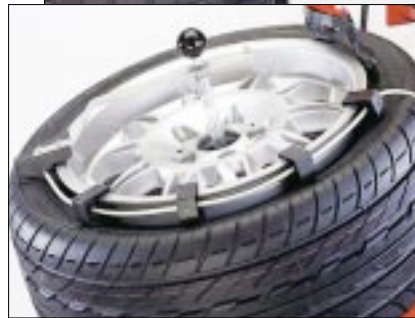
Bead Depressor "Tail" aids in positioning low-profile tires down into drop-center for mounting and demounting.
