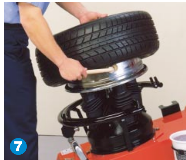
Bead Depressor "Tail" aids in positioning low-profile tires down into drop-center for mounting and demounting.
