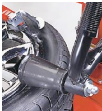
Pushes tough tires down into the drop-center for quicker, easier mounting.
