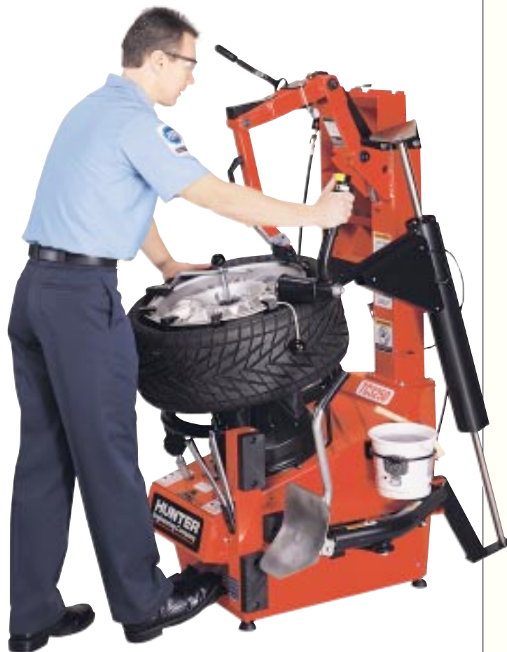
Pushes tough tires down into the drop-center for quicker, easier mounting.
