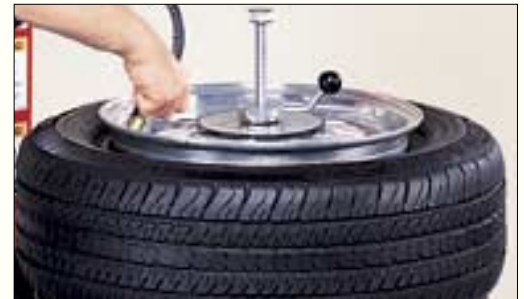
Rim Securing Device secures wheel to clamping table in case of tire failure during inflation.
